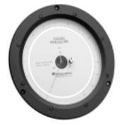
For routine test and production uses, this capsule-type gauge offers an acceptable balance among size, readability, accuracy, and price. Available in 18 standard ranges (including vacuum and compound ranges), the Series 300 is convenient to use. High differential pressure is applied to the capsule; low pressure to the case. Maximum static (case) pressure is 15 psig. A built-in overpressure relief valve protects the case.
